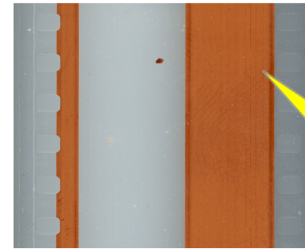
Part coated Magnetic film with 100 mil and balance stripe
