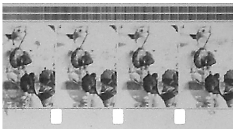
16mm with twin Variable Density tracks
