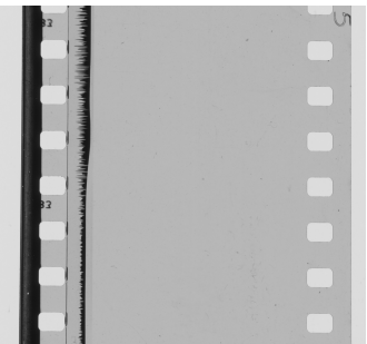
Unilateral track with shutter noise reduction
